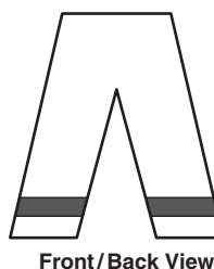
FIGURE 7.2.4 Minimum Required Structural Firefighting Trouser Trim Patterns.
