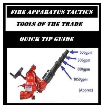
It is interesting to see deck guns/ stacked tips being used at massive fires where they have lots of water and firefighters don't remove the extra stacked tips. The difference in reach is small but the flow is doubled from the small to the large. Unless you are specifically trying to have less water application (weight/collapse implications on a fire damaged building) use the big tip!
