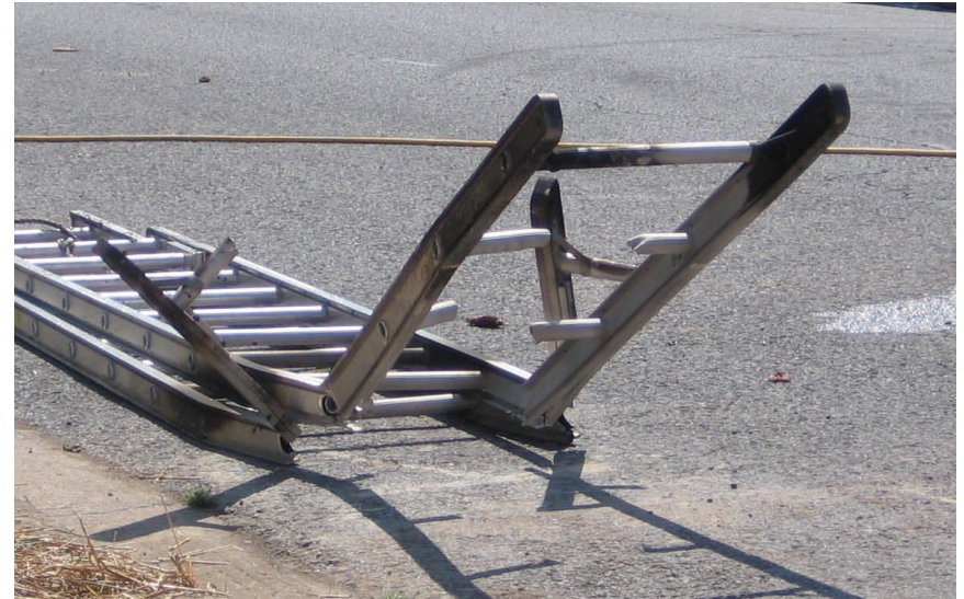
The result of fire venting from a window impinging on a 24' aluminum ground ladder.
