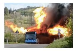
Alternative fuel buses are becoming more common on the streets in our communities. Buses using Compressed Natural Gas (CNG) have the storage tanks mounted on the roof of the bus. If the bus strikes a bridge or other low hanging obstacle, it may cause failure of the cylinder.
