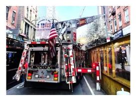
Will the length of the soft-suction from your front intake continue to reach the hydrant now? You may need a longer length of LDH to make the connection. What about the building fire department connections (FDC), are they now blocked or hidden? Also apparatus equipped with "barrier clearance doors" as opposed to full length doors enable safer egress from the cab with tools and SCBA.
